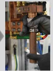
Easily retrofit your existing adapter assembly (left) with the Quick Change Electrode (right).
